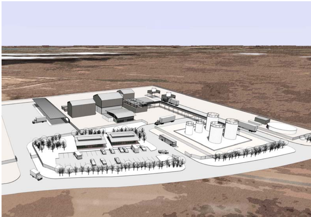
Figure 5-1: Typical layout for 200-tpd pyrolysis plant including feed receivals, preparation and storage, pyrolysis, product storage and associated facilities, courtesy Renewable Oil Corporation Pty Ltd
